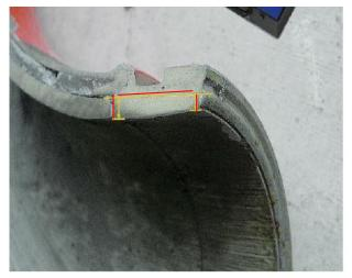
Fig. 32: Measuring pipe wear: wall thickness measuring units for two-layer lines (le.) and single-layer lines (ri.)
